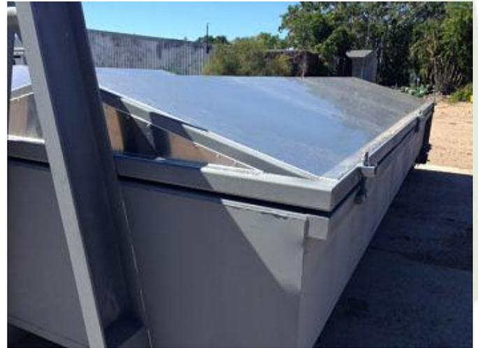
Council manufactured its own purpose built RORO containers to hold the waste which are fully sealed and are now in service. The movement of the biosolid containers will be scheduled to coincide with movements of waste or recycling in a truck and dog trailer combination to ensure efficiency of operations.
