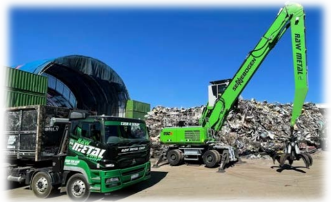
One of the fleet trucks with a Sennebogen 830 excavator and 5 finger-grab
