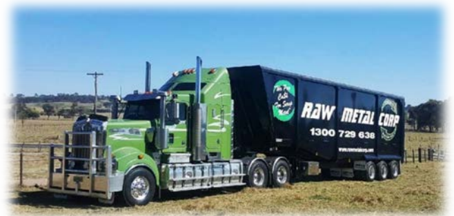
A 90m 3 Tefco trailer for hauling the scrap metal back to our yards
