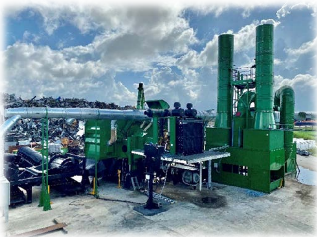
Bonfiglioli Hammer Mill metal shredder in our Mackay yard capable of processing 25 tonnes of scrap metal per hour ready for exporting.
